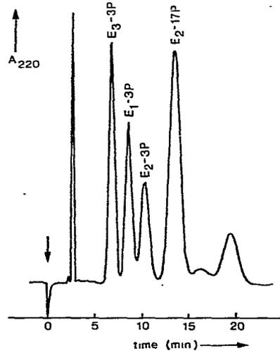
Fig. 9. Separation of an estrogen glucuronide mixture. Phase system: B 300, 13  $\mu$ m; 0.025 M perchlorate + 0.01 M phosphate, pH 7.0. Temperature, 25°; pressure, 16 bar.
