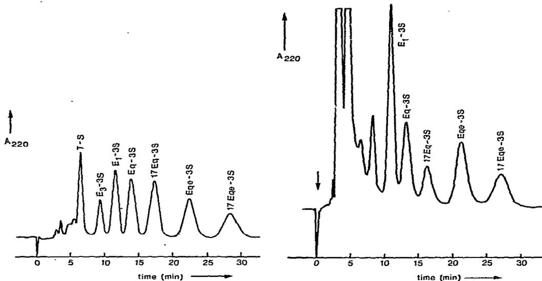
Fig. 11. Separation of estrogen sulphates. Phase system: ET 41, 11  $\mu$ m; 0.25 M perchlorate + 0.01 M phosphate, pH 8.5. Temperature, 70°; pressure, 30 bar.
