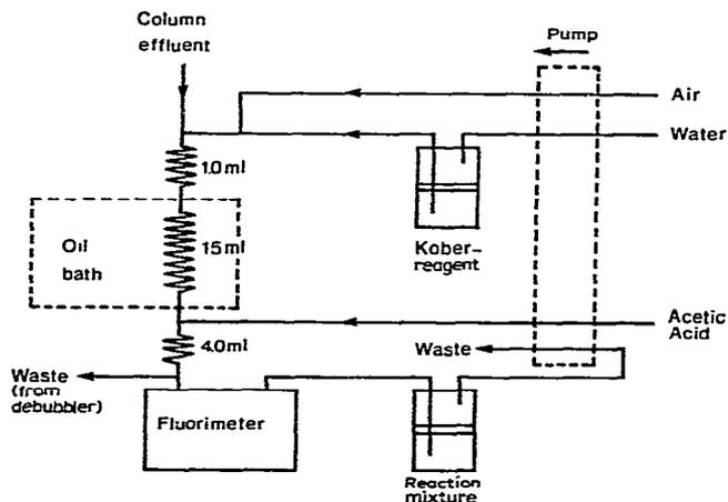
Fig. 1. Schematic diagram of the gas-segmented-flow reaction detector.
