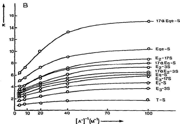
Fig. 6. Dependence of the capacity ratio,  $\kappa_i$ , on the inverse of the eluent anion concentration,  $[A^-]^{-1}$ . A, 17 $\beta$ -Estradiol conjugates. Phase system: B 300, 19  $\mu$ m; perchlorate + 0.01 M phosphate, pH 6.8; 70°. B, Estrogen sulphates. Phase system: B 300, 19  $\mu$ m, perchlorate + 0.01 M phosphate, pH 6.8; 70°.
