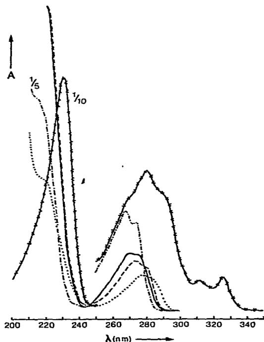
Fig. 2. UV spectra of estrogen conjugates in deionized water. -V-V-V-, 17 $\alpha$  E<sub>qe</sub>-3S; ---, E<sub>2</sub>-3G; ·····, E<sub>2</sub>-3S; -·-·-·, E<sub>2</sub>-17G; ———, E<sub>2</sub>-3P.
