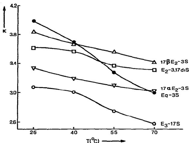
Fig. 8. Dependence of the capacity ratio on temperature for some estrogen sulphates. Phase system: ET 41, 11  $\mu$ m; 0.25 M perchlorate + 0.01 M phosphate, pH 8.5.
