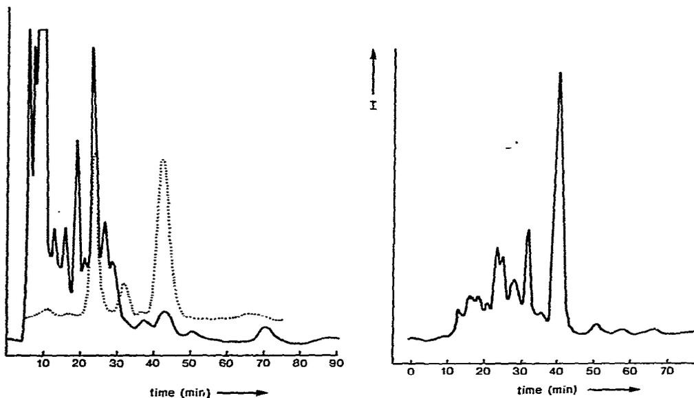
Fig. 13. Chromatogram of a methanolic XAD-2 extract of human pregnancy urine. Solid line, absorbance at 220 nm; dotted line, chromatogram obtained by off-line batch determination of estrogenic material. Phase system: B 300, 11  $\mu$ m; 0.025 M perchlorate + 0.01 M phosphate, pH 6.8. Temperature, 70°; pressure, 20 bar.
