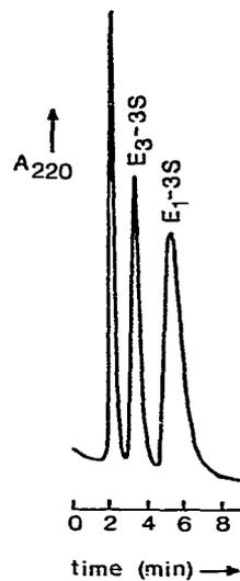
Fig. 3. Separation of four steroid conjugates on Cellex T, 14  $\mu\text{m}$ . Eluent: 0.25  $M$  perchlorate + 0.01  $M$  phosphate, pH 6.8. Temperature: 75°.
